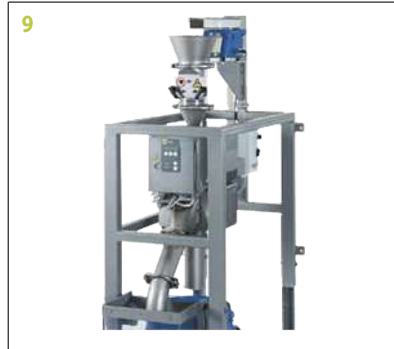
PRESEP Metal Separator Designed for highly contaminated material; neodymium magnets first separate all metallic contaminants before the metal separator removes all non magnetic contamination.
