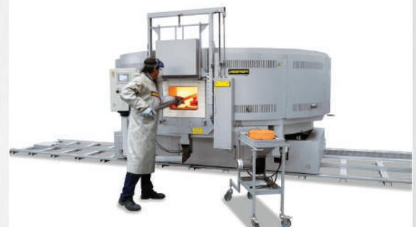
**ROTARY HEARTH FURNACE UP TO 1300°C WITH AND WITHOUT AIR CIRCULATION**
