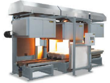
**LIFT-TOP OR LIFT-BOTTOM FURNACE WITH WIRE HEATING UP TO 1400°C, ALSO AS COMBI FURNACE FOR DEBINDING AND SINTERING IN ONE PROCESS**
