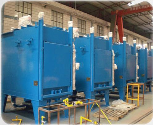
FOR APPLICATION OF RELIEVE THE INTERNAL STRESSES AND REDUCE BRITTLINESS OF METAL PARTS AFTER HARDENING.
