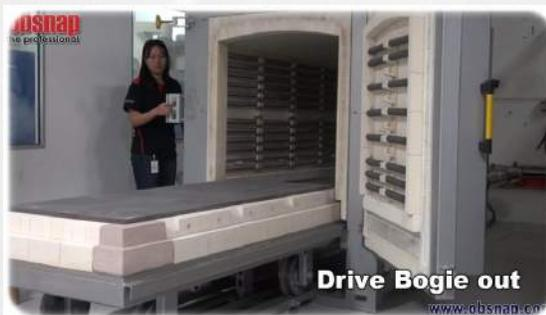
BOGIES WITH FLANGED WHEELS RUNNING ON RAILS FOR EASY AND PRECISE MOVEMENT OF HEAVY LOADS
