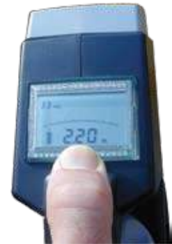
LCD meter display signal strength, operation mode, depth and battery condition.
