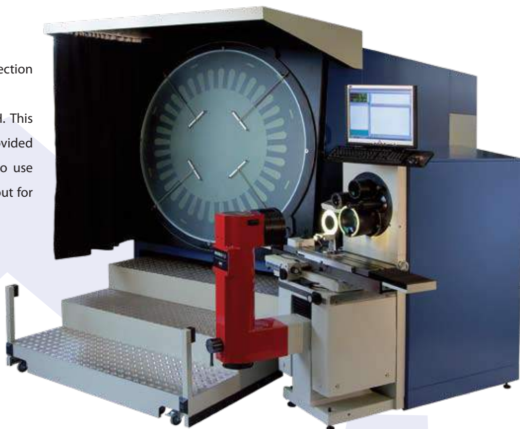
SIRIUS with 500mm screen diameter, horizontal projection system, large and sturdy front worktable with powered displacements of either 300 x 200mm or 710 x 200mm.
