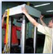
Compression tester was being assembled back after repair was completed.
