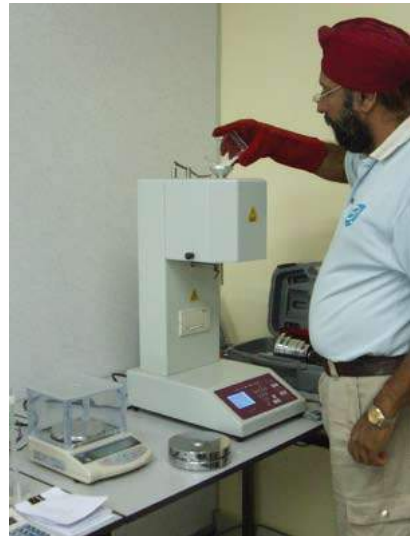
Measuring Melt flow index of plastic raw material by our customer in plastic industries
