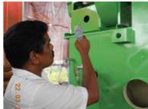
Temperature measurement with an Infrared thermometer
