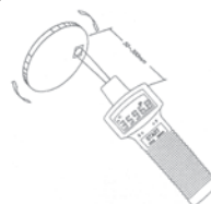
1. Point the photoelectric probe at the object. Measurement of Rotating Speed (rpm, rps)
